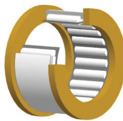
(W) Roller Bearing with Thrust Washers
